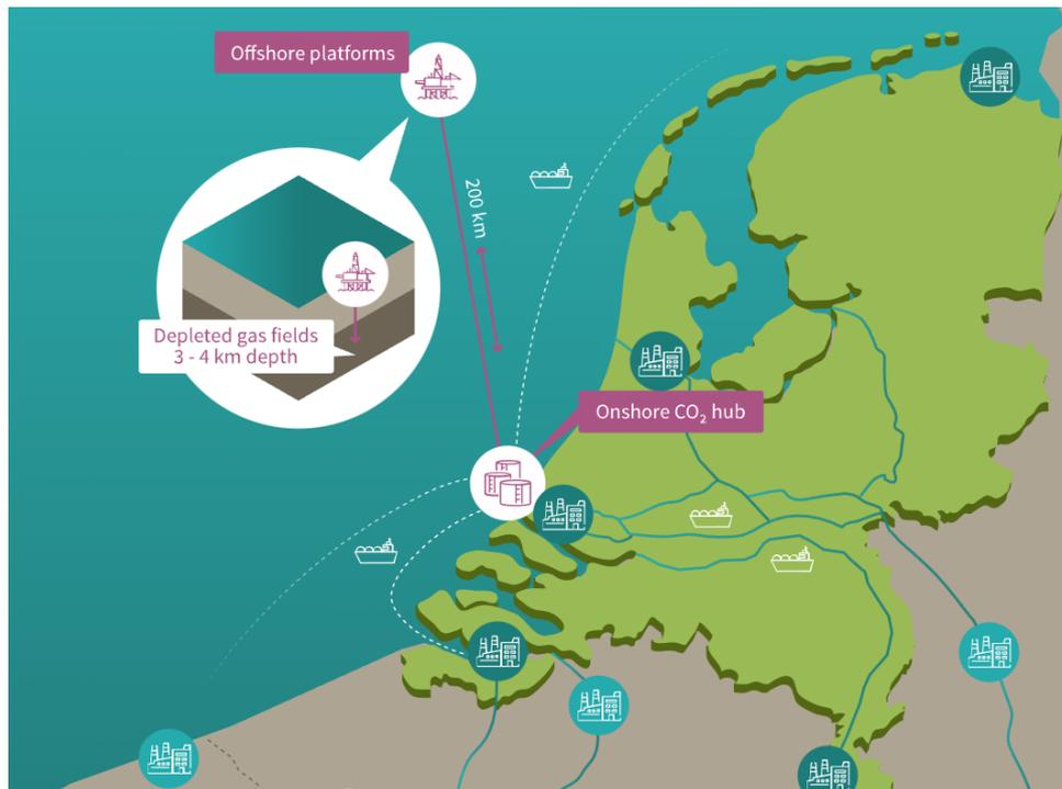
Figure 28. Illustration of the Aramis pipeline and the approximate location of the offshore CCS locations (<https://www.aramis-ccs.com/project>).
