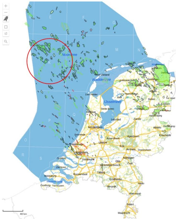
Figure 29. Map of the Netherlands onshore and offshore, with existing gas (green) and oil (red) fields and the area of interest for the Aramis CCS project (red circle). (<https://www.nlog.nl/kaart-boringen>).
